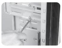
B-3. Secure the card reader with the screws provided or the case 3.5" mounting system.
